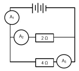
How will the readings on ammeters A<sub>1</sub>, A<sub>2</sub> and A<sub>3</sub> compare with each other?
